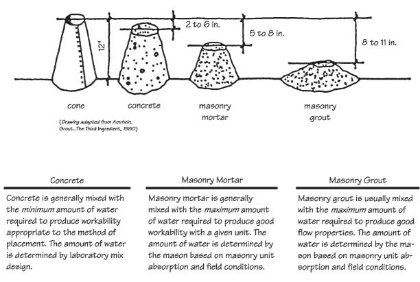
Figure 6-11 Relative consistency of concrete, mortar, and grout as measured by slump test.
